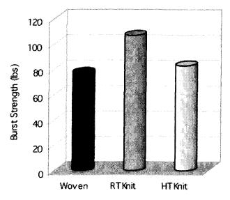
Figure 10. Comparison of ball-burst strengths of the ePTFE fabrics.
