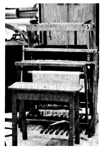
Figure 8. Hand loom used for production of woven ePTFE fabrics
