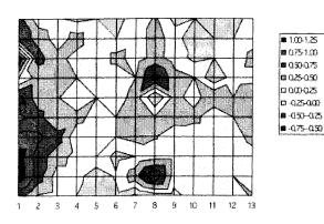
Figure 6. Calculated warp direction tensile strains in beige 4/4 fabric.
