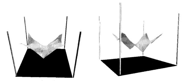
Figure 5. Meshworks visualization of a 4/4 configuration knitted fabric constructed from empirical digitization of the structure.
