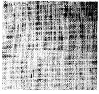
Figure 9. Hand-woven plain weave using ePTFE continuous filament yarn.
